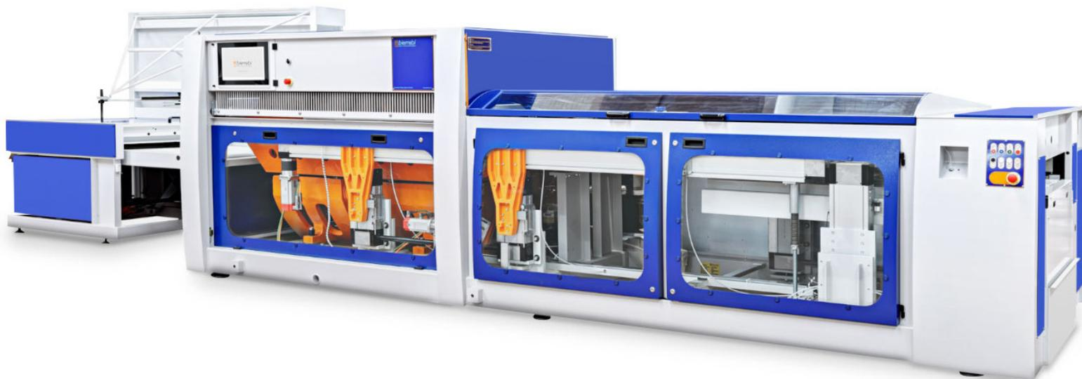
The OF Line is a modular cutting system that can be equipped with a different number of feeders and with different die cutting punches depending on specific customer requirements. The main benefits are:
